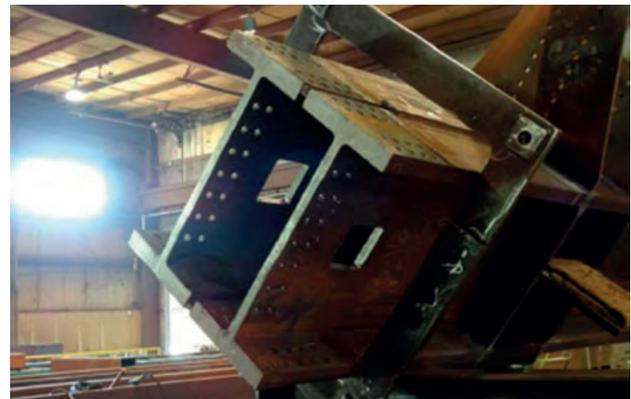
Two heavy sections welded together
